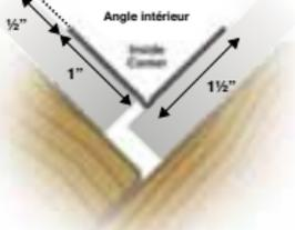
DESIGNED FOR STRAIGHTENING COMMON IRREGULARITIES IN VAULTED CEILINGS AND COFFERS
