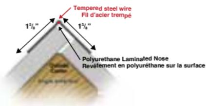
DESIGNED TO ELIMINATE FLAT SPOTS IN CURVED APPLICATIONS
