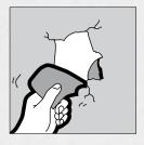
b. Apply a skim coat of drywall compound with a drywall finishing knife to damaged area and feather to get a smooth finish. Let dry and apply second coat if necessary. Sand and prime when dry.
