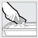
Keep the blade clean, especially of dried bits of compound, to avoid leaving scratches in the wet drywall compound as you draw the knife over it. Discard any compound containing dried bits of material. Clean blade by drawing it over edge of pan.
