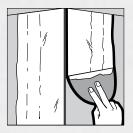
Using a 150 mm (6 in.) taping knife for outside corners (100 mm [4 in.] for inside corners), apply another coat of drywall compound. Keep this coat as smooth as possible. Feather out 125 mm to 150 mm (5 in. to 6 in.) from the nose of the trim on each side for outside corners 25 mm (1 in.) past previous coat for inside corners. Let dry. Sand sides lightly where needed.
