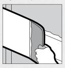
Apply pressure to knife edge farthest from the joint and lift the other edge just slightly above surface. Draw knife down joint. Repeat for opposite edge. This technique is called feathering. Drywall compound should extend beyond first coat for a total width of 180 mm or 200 mm (7 in. or 8 in.).
