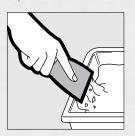
While embedding tape, draw the knife slowly along the length of the tape to provide an even distribution of drywall compound. Don't worry about a few grooves or streaks in the drywall compound. They will be covered over in the subsequent coats.
