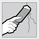
c. To repair a popped nail, drive and dimple new nail 38 mm (1-1/2 in.) from popped nail. Drive and dimple popped nail. Cover with drywall compound. Sand and prime when dry.
