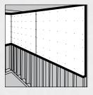
Apply lower row of panels so tapered edges meet with those of top row. Vertical joints should be staggered. Avoid vertical joints directly above or below a window, door or other opening for best decorating results.
