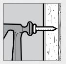
Double-nailing reduces the likelihood of nail pops. It is highly recommended for ceilings. Drive first nails 300 mm (12 in.) o.c. along framing in the field of the board and second nails about 50 mm (2 in.) from the first. Fasten the perimeter 180 mm (7 in.) o.c. for ceilings and 200 mm (8 in.) o.c. for walls.
