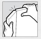
Use utility knife with sharp blade for scoring. Complete cutting by running knife through back paper for the length of the panel and snapping back to face.
