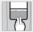
Apply a 180 mm or 200 mm (7 in. or 8 in.) coat of drywall compound to each side of butt joints and feather. Compound should extend beyond first coat for a total width of 350 mm (14 in.).
