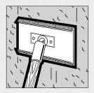
Before applying the final coat, check to see if tapered joints are level with surface. Hold the 250 mm (10 in.) blade across the joint, straight out from the wall. If the blade can be rocked across the joint, the joint is crowned. It must be hidden by feathering the final coat out as far as possible.
