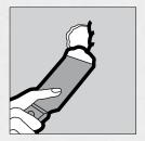
c. Crisscross two or three strips of joint tape over opening and embed tape in drywall compound. Let harden.
