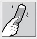
b. To repair a small hole or crack, trim any loose pieces from the damaged area and wipe it clean. Fill with drywall compound, using a putty knife. Let harden. Add second coat if necessary. Sand and prime when dry.
