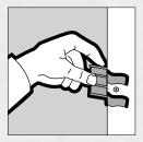
c. Measure and cut new drywall panel section to fit damaged area. Screw through new drywall into each drywall repair clip. Screw into drywall, positioning screw opposite screw holding clip and about 20 mm (3/4 in.) from edge.
