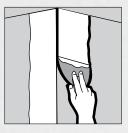
Place trim on wall and press into position. Corner bead should be aligned tight to ceiling. Embed trim by running the knife over it with even pressure at a 45° angle.
