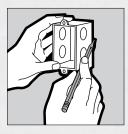
Cut with keyhole saw, jab saw or rotozip. Wear a dust mask if excessive dust is produced and the area cannot be ventilated.
